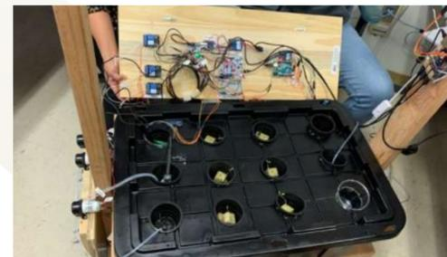
Figure 3: (above) hydroponic circuitry and seedling setup
